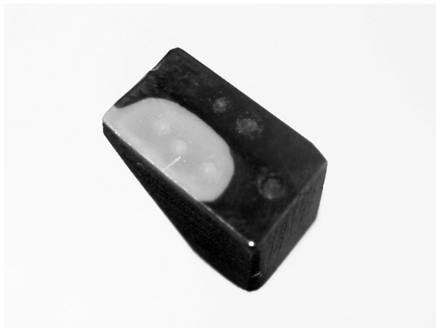
Figure 6-4: Sample LR3; exhibiting the extremely well-defined interface between the grey and black regions.
