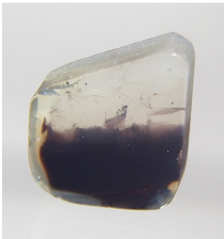
Figure 6-5: Detail of interfacial region of Sample LR1. Note the fluid-like appearance of the interfacial region between the two bands.
